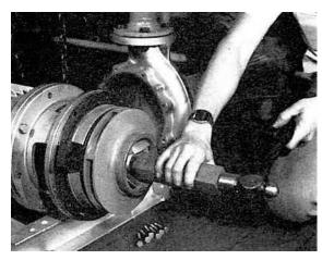
3. Remove the bell housing to backplate bolts and remove the backplate.
