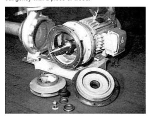
A pump which has become worn in the body or impeller may be repaired by fitting bronze wear rings. These rings, with full instructions for machining the pump parts and fitting rings are obtainable from the nearest Southern Cross Dealer.
