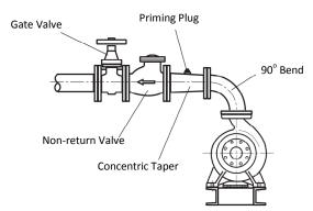
To avoid the formation of air pockets in the discharge piping (ie. at the high points), vent cocks must be placed to expel any accumulation of air which may affect the discharge capacity of the pump.
