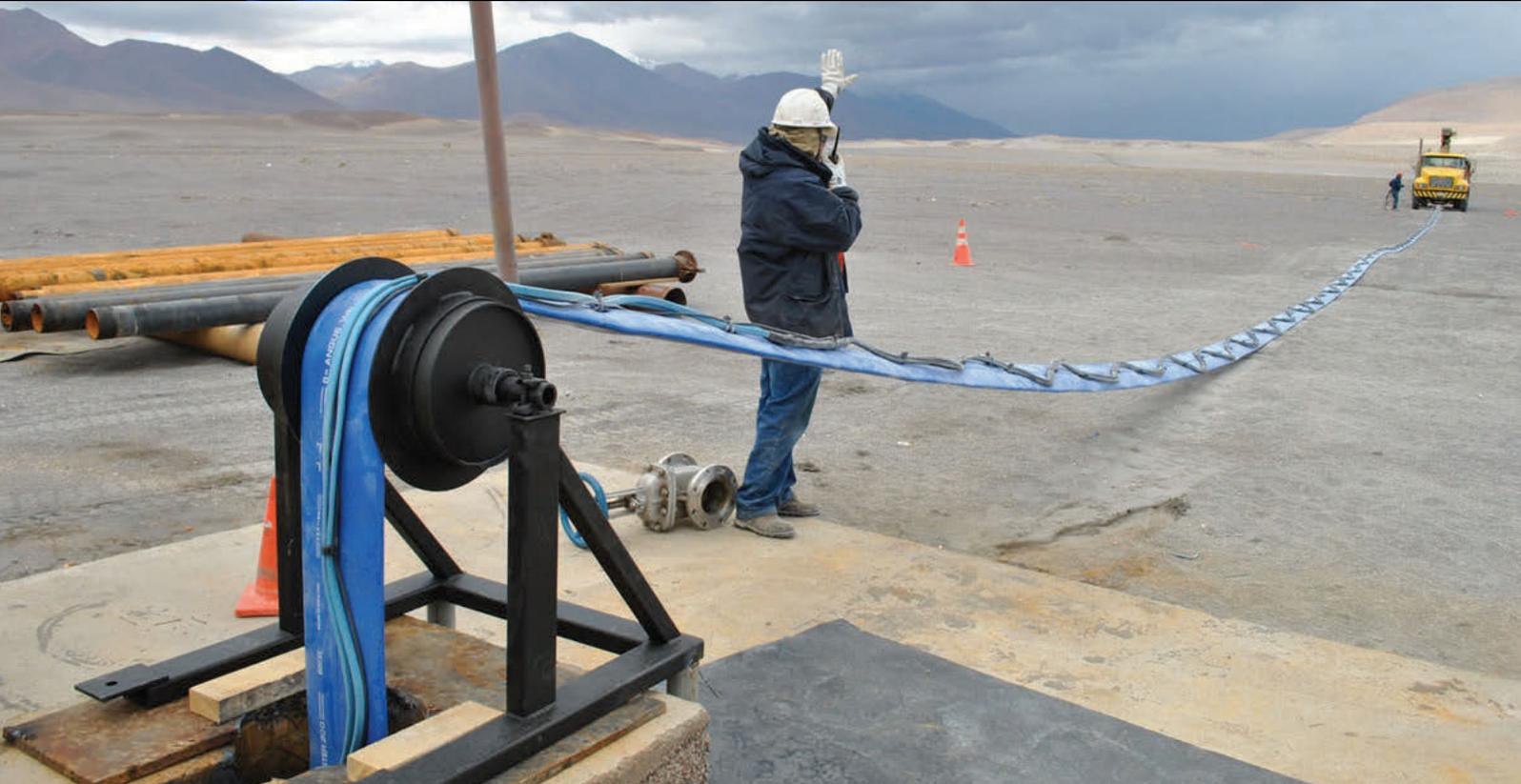
**The Wellmaster range is the Flexible Rising Main System for all types of ground water extraction and well monitoring operations.**
